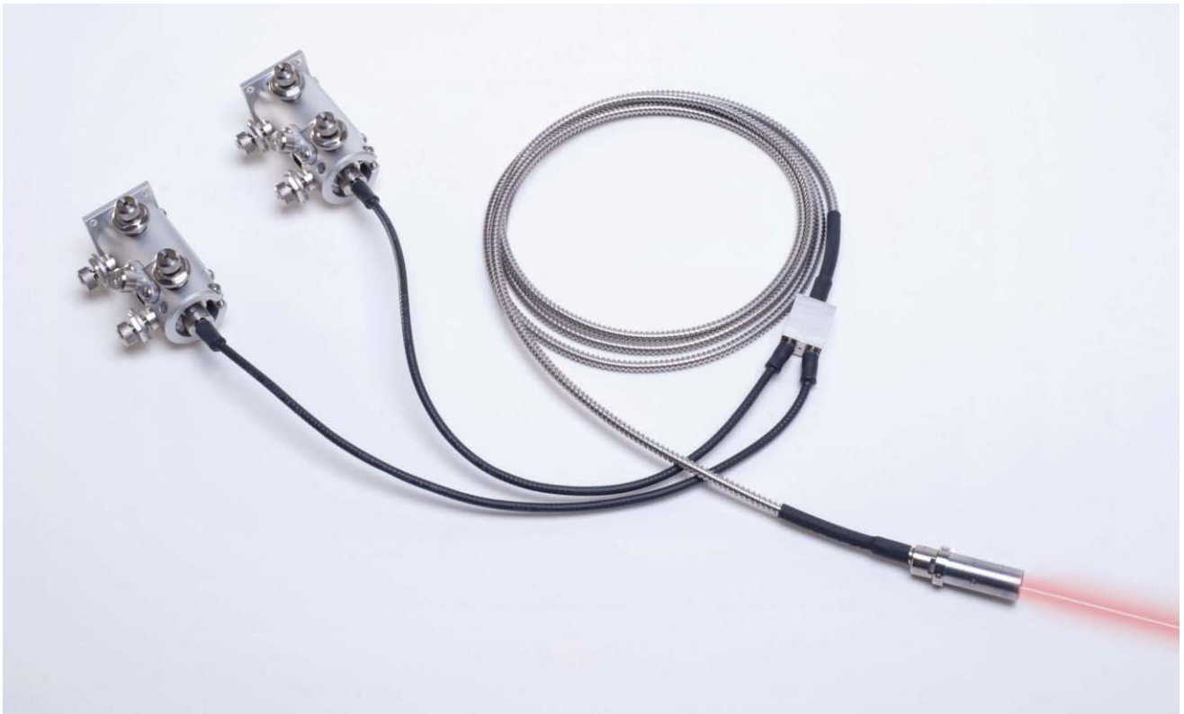
FIGURE 2. The two-line kineFLEX-Hydra fiber delivery system includes the integrated output beam-shaping optics that shape parallel and collinear beams. The system includes two kineMATIX manipulators, one at each input end for aligning and attaching the fibers to the individual lasers. By choosing to decouple the laser from the fiber at the laser side, the fiber can remain in situ and the output end can remain buried within the instrument when the laser is replaced at end of life. This then allows the laser to be located in a more convenient location for servicing and heat dissipation.
